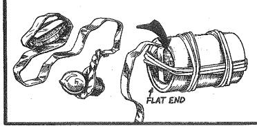
Slide the rubber band off the bump on your dry cell. Check to see that the bulb lights.
